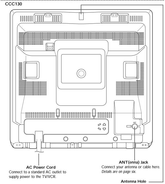
Connect the stem of an indoor antenna here. Details are on page six.
